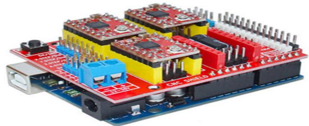
Fig 9 A4988 can also be interfaced with Arduino through CNC Shield
